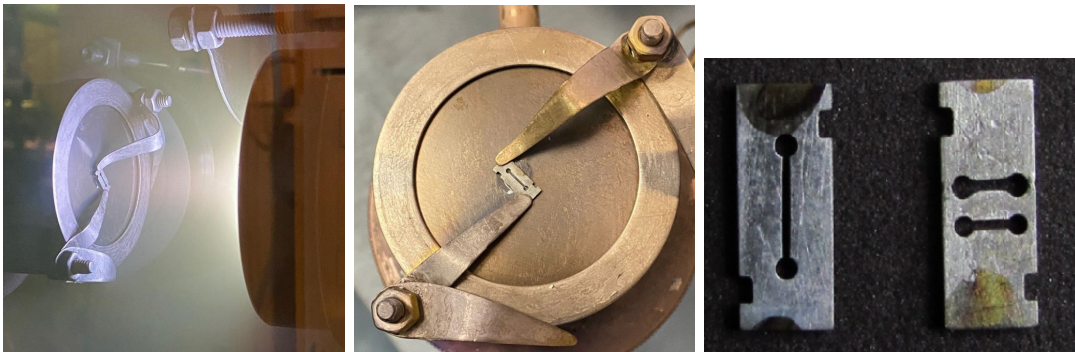
Figure 2.5: Images depicting the sputtering plasma glow (left), a loaded substrate with the NbN mask (middle) and the shadow masks for NbN and Ag (right).
